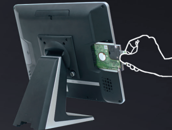
HDD / SSD easily accessible
